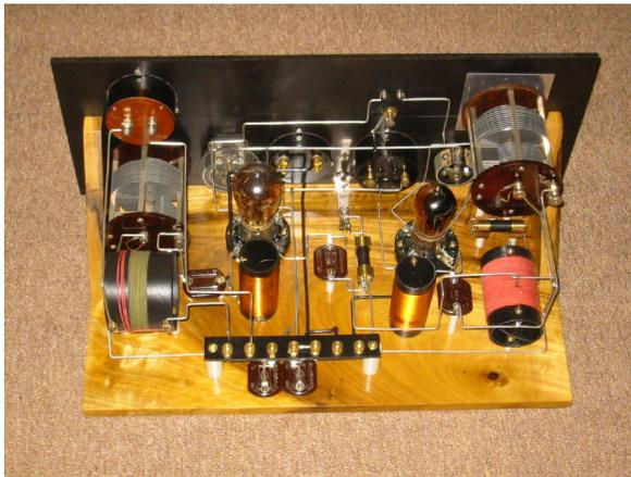
◀ **Behind the MOPA panel. Ladder line feeds a 160 meter dipole as the hat of Brian’s Marconi T transmitting antenna.**
